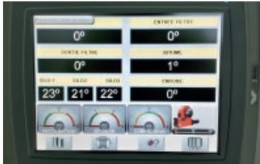
Terminal tactile HMI (Human Machine Interface).
