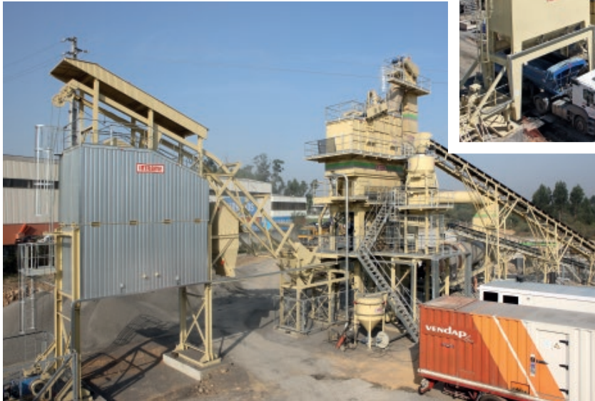
100 t silo installed in a M-280 asphalt plant.
