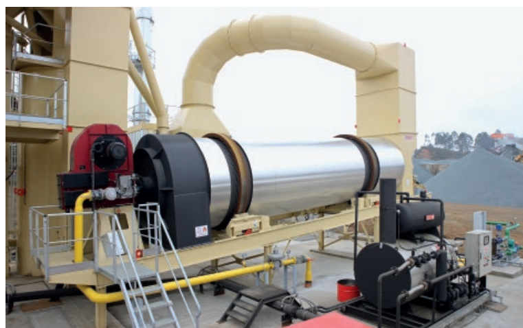
RM-280 dryer. Of high efficiency. Equipped with a high efficiency burner that complies with the strictest international environmental regulations. Also, in the forefront is shown the hot oil heater of high energetic efficiency.
