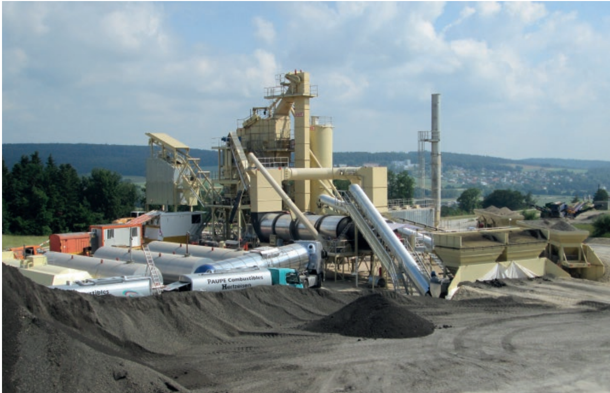
Hot process recycling equipment RC-120 installed in a M-280 asphalt plant (Switzerland).
