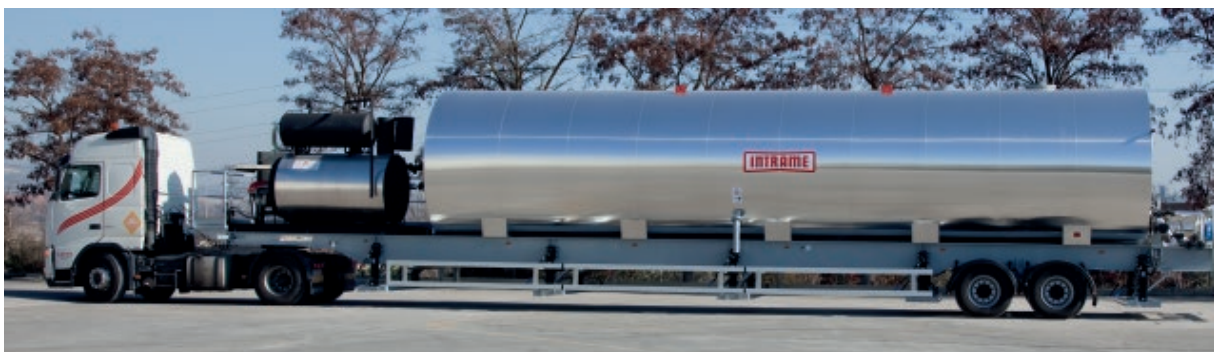
Mobile tank on wheels incorporating heater.
