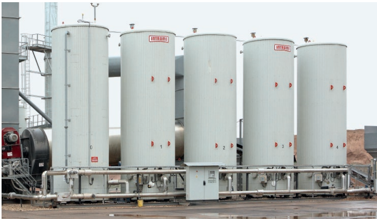
Electrically heated storage tanks in InNOVA 320 plant (Poland).
