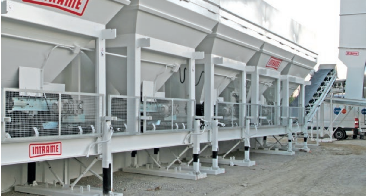
Detail of cold feeders load distributors.
