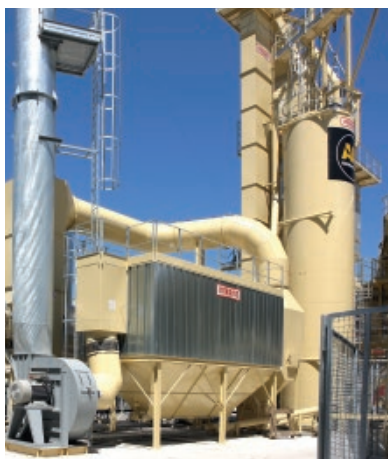
View of a bag house and a double silo for recovered dust and added filler in a RM-280.
