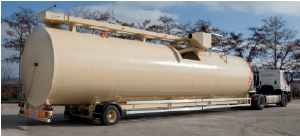
Double silo for recovered dust and added filler.
