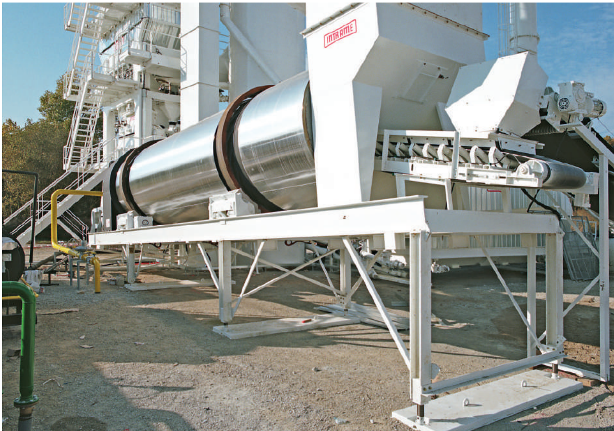
Detail of dryer's load distributors.
