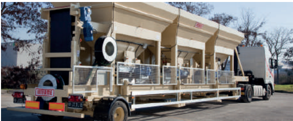
Cold feeders second unit.
