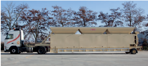
Cold feeders first unit.
