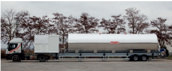
Second tank with control cabin.
