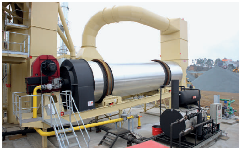
RM-280 dryer. Of high efficiency. Equipped with a high efficiency burner that complies with the strictest international environmental regulations. Also, in the forefront is shown the hot oil heater of high energetic efficiency.
