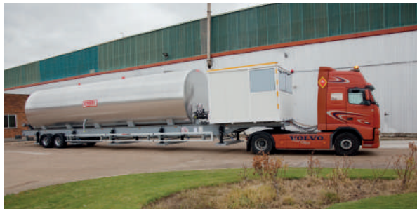
Storage tank with control cabin.
