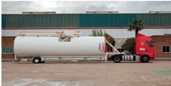
Double silo for recovered dust and added filler.
