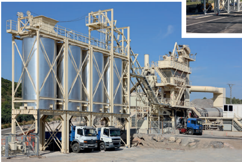
Battery of four silos, 85 t each, loaded through a horizontal displacement hopper that collects the hot mix from the mixer by means of an elevating skip. Each silo is equipped with a weighing system to control truck loading.
