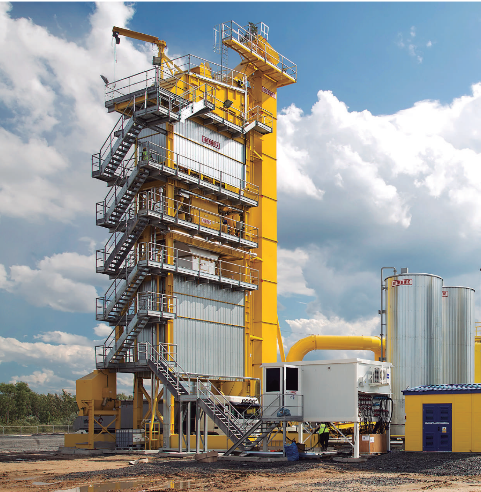
M-200 InNOVA asphalt plant.
