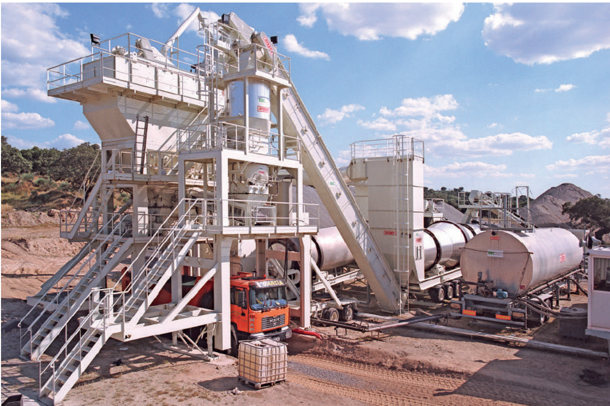
Hot process recycling equipment RC-80 installed in a UM-200 asphalt plant (Spain).
