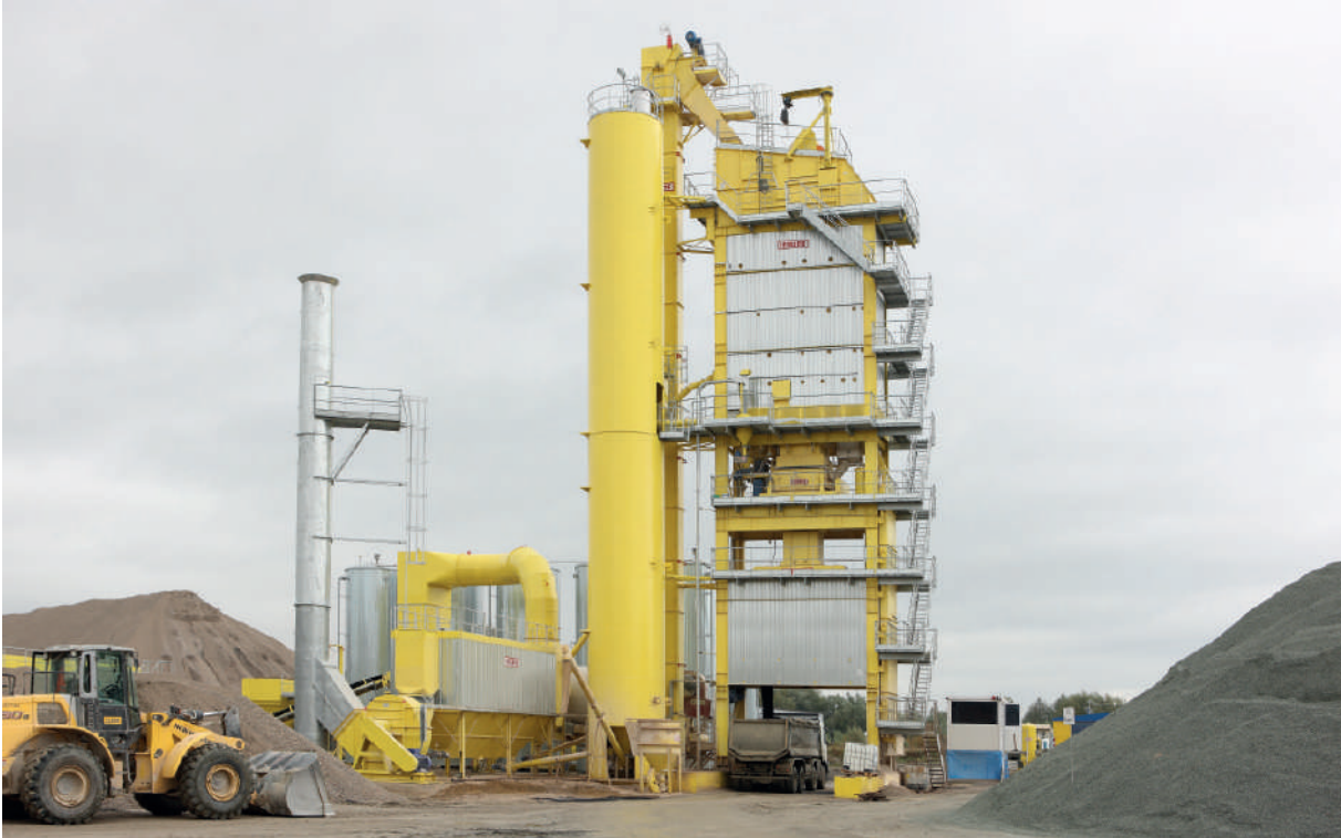
320 t/h asphalt plant (Poland). With InNOVA-G mixing tower. Equipped with 160 t capacity hot bins and 81 t capacity hot mix storage silo. 4.500 kg mixer.
