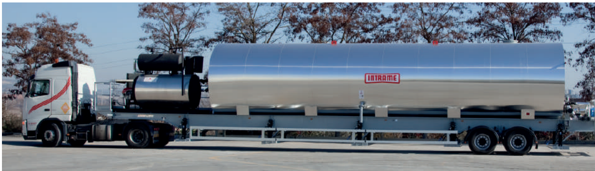
Mobile tank on wheels incorporating heater.
