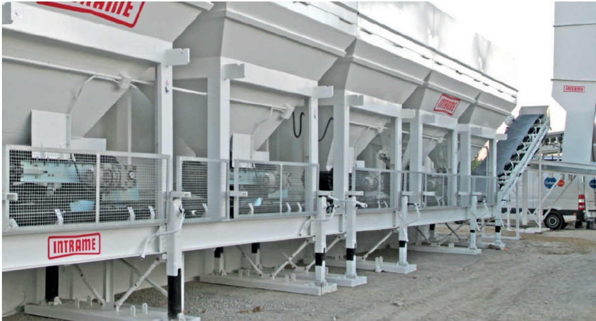
Detail of cold feeders load distributors.
