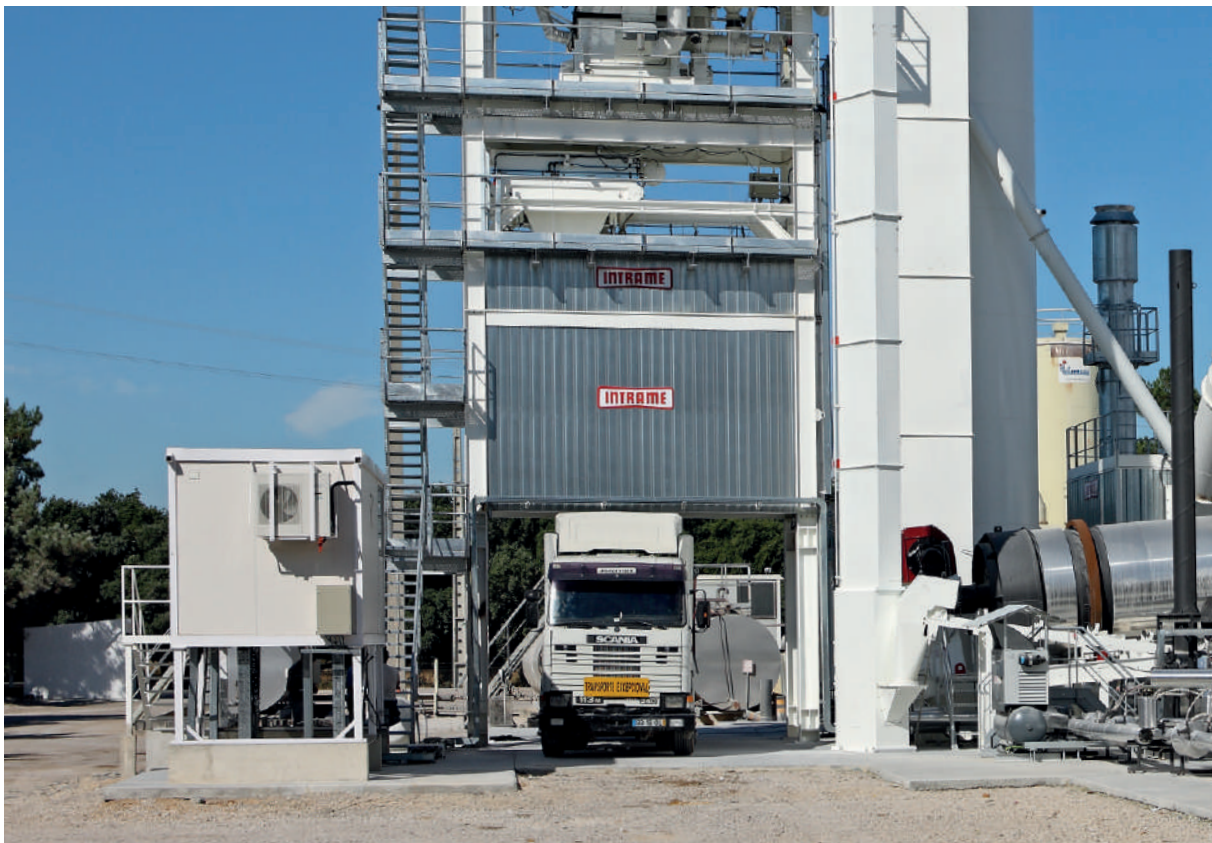
Plant with silo under the mixer. Loading by gravity through a wheel mounted hopper with horizontal displacement, thus allowing the installation of additional silos.
