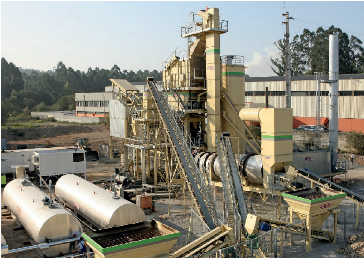
Double line recycling equipment.
